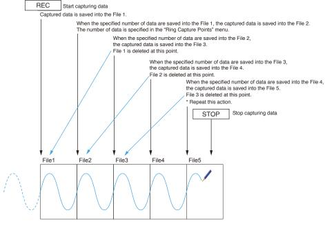
When capturing is stopped at the STOP point in the above, the File4 and the File 5 are remained. These files are consolidated into one file and it is saved. Then the ring catpuer is completed.
