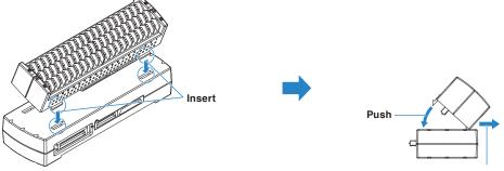
\* For the withstand high-voltage high-precision terminal (B-565), push it in while pulling it toward you.
