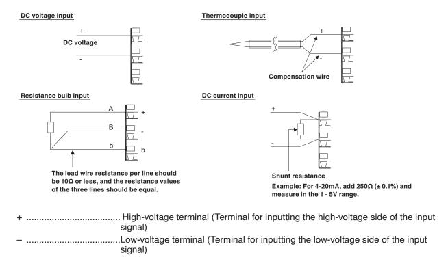
b ......Dedicated terminal used to connect the resistance bulb.
