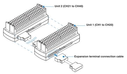
(3) Connect the other end the expansion terminal connection cable to the terminal connector on the GLT400. Push the expansion terminal connection cable until it is completely locked.
