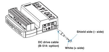
(3) Connect the DC input side to the DC power supply.
