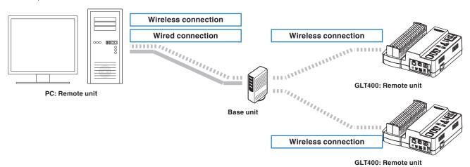
(2) Connect to the wireless LAN base unit of midi LOGGER GLT400
