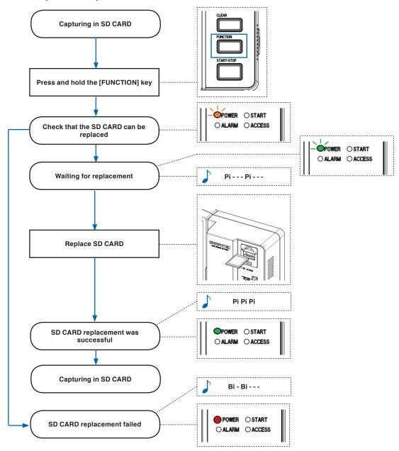
If an error occurs when replacing the SD CARD, the POWER LED is lit in red, so insert a writable SD CARD.
