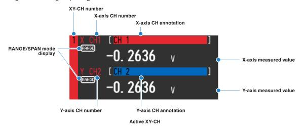
RANGE/SPAN mode display T-axis measured value Y-axis measured value
