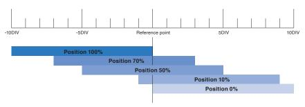
As shown in the figure above, the display range moves 10DIV area in parallel through the XY position setting. XY position setting is set only for XY graph.
