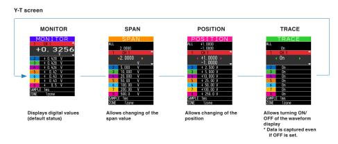
Use [CH SELECT] key or the  $\blacktriangle$   $\blacktriangledown$  keys to move on the CH.
