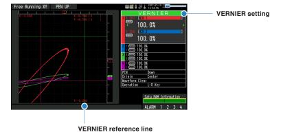
The VERNIER reference line is displayed at the position of 5DIV from the position reference point when the VERNIER is set to 100%. When the VERNIER is set to 80%, it is displayed at the position of 4DIV from the position reference line (80% position compared with 100%).
