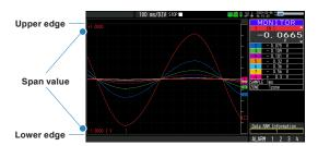
The span value is displayed as the scale display of the CH set to the active CH.
