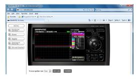
Remote key operation....... This device can be remotely operated.
