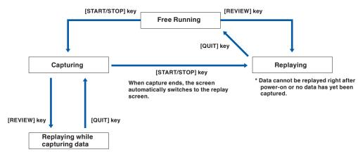
The operation modes are described using the Y-T + Digital display screen.
