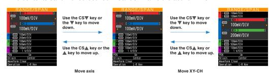
Change the setting contents of XY-CH/axis selected with the ◀▶ keys.
