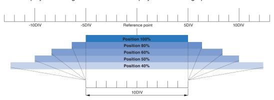
When the Vernier is set to 100%, it magnifies equally along the axis. Therefore the waveform display reflects the Vernier setting magnification.
