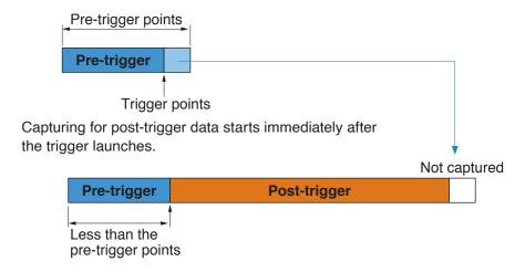
The total data after capturing is less due to the uncaptured pre-trigger point.
