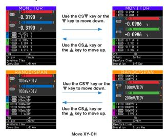
Change the setting contents of X-axis for XY-CH selected with the ◀▶ keys.
