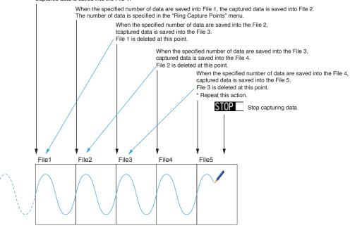
When recording is stopped at the STOP point in the above, File 4 and File 5 remains in the memory. These files are consolidated into one file. Ring capturing completes after combing the files.
