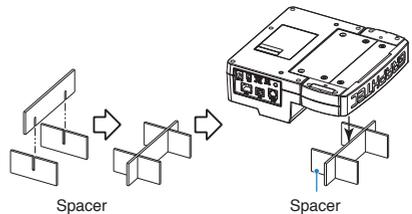
4. Turn the direct-connected GLT400 over and place it on the spacer as shown in the figure. Tighten the screws without rattling. (When connecting multiple GLT400s, ensure a height of 33.5 mm without rattling.)
