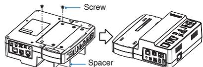
5. Insert the terminal into the terminal base.
