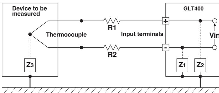
Ex 2: Connect the GLT400's GND to the GND of the device to be measured.
