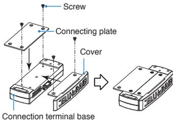
2. Direct-connect the terminal base to the GLT400. It is recommended to direct-connect them on a flat desk. Then, connect the connector cover to the expansion terminal base.
