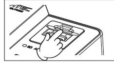
1. The SD CARD is released by pushing gently on the SD CARD. Then, pull to remove the SD CARD.
