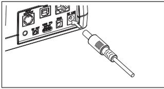
Connect the DC output of the AC adapter to the connector marked "DC LINE" on the GLT400.
