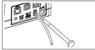
Connect the ground cable to the GLT400 while pushing the button above the GND terminal with a flathead screwdriver. Connect other end of the cable to ground.
