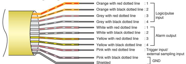
\* The B-513 input/output cable for GL (option) is required for connecting external input/output. (Logic/pulse input, alarm output, trigger input)
