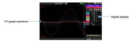
Using Y-T graph waveform on the left side and digital value on the right side, currently measured values can be monitored.
