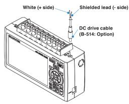
(3) Connect the DC input side to the DC power supply.
