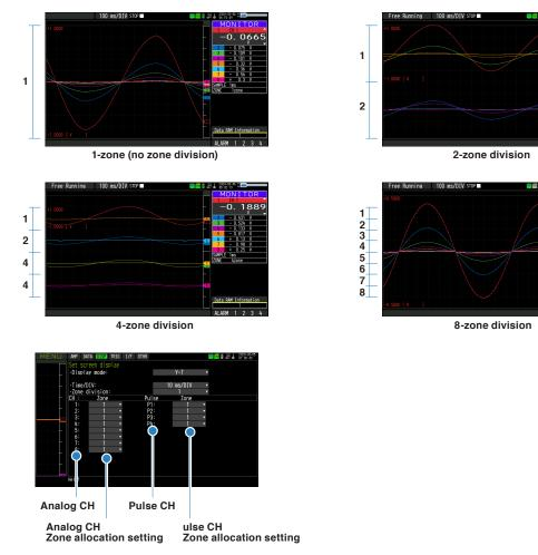
Analog CH and pulse CH can be freely assigned to each zone.
