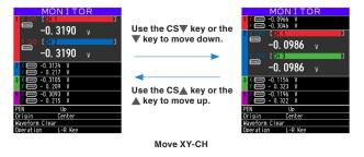
In addition to the above setting, use CS key or the  $\blacktriangle \forall$  keys move the axis. Then, press the same direction key to move between XY-CH channels.
