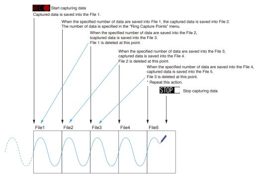
When recording is stopped at the STOP point in the above, File 4 and File 5 remains in the memory. These files are consolidated into one file. Ring capturing completes after combing the files.
