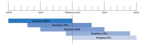
As shown in the figure above, the display range moves 10DIV area in parallel through the XY position setting.
