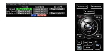
[FUNC] key can be set according to each screen mode (Y-T/logging/XY) and operating status (free running/ capturing/replaying) respectively.
