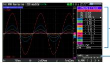
Displays the voltage at a point indicated by Cursor A or B or the selected cursor.
