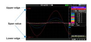
The span value is displayed as the scale display of the CH set to the active CH.
