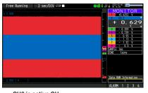
CH2 is active CH. The waveform of CH2 is displayed on the top, so you can visually recognized it.
