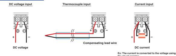
the shunt register. For 4 to 20mA current input, install 250 ohms (0.1%) resister for converting 1 to 5V.
