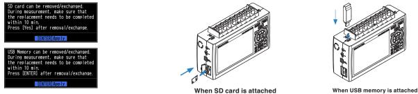
(5) Make sure that the device access indicator turns green and then press [ENTER] key. For access to device access indicator, refer to "3.1 Window names and functions".
