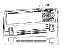
(4) Remove the body completely from the Rubber Protector.
