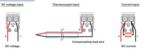
Ex: The current is converted to the voltage using the shunt register. For 4 to 20mA current input, install 250 ohms (0.1%) resister for converting 1 to 5V.
