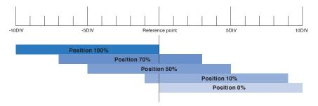
As shown in the above figure, the display range moves in parallel with 10DIV area with the XY position setting.
