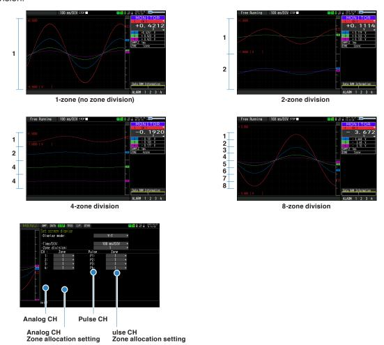
Analog CH and pulse CH can be freely assigned to each zone.
