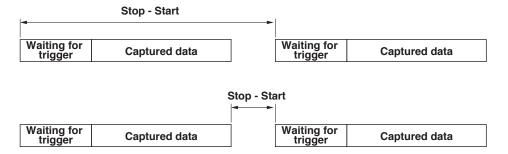
When the time interval between start and stop is set and the set time interval has passed at the end of the capturing, repeat operation starts immediately.
