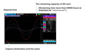
The captured data is saved in the Internal RAM, internal memory, SD card or USB memory during data capture.
