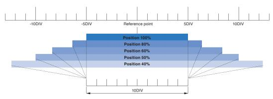
When the VERNIER is set to 100%, it becomes an equal magnification. Therefore the waveform display is shrunk by the VERNIER setting magnification.
