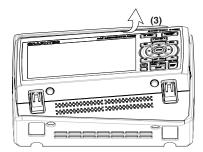
(4) Remove the body completely from the Rubber Protector.
