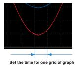
The range of the Time/DIV value that can set depends on the sampling interval setting.
