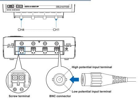
The screw terminal and the BNC connector are internally connected. You can measure with either input.
