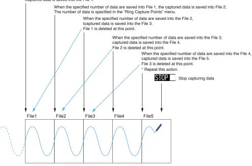
When recording is stopped at the STOP point in the above, File 4 and File 5 remains in the memory. These files are consolidated into one file. Ring capturing completes after combing the files.
