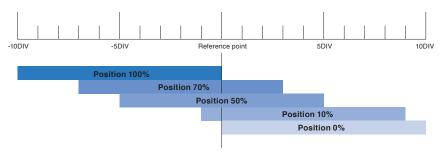
As shown in the figure above, the display range moves 10DIV area in parallel through the XY position setting.
