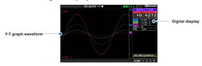
Using Y-T graph waveform on the left side and digital value on the right side, currently measured values can be monitored.
