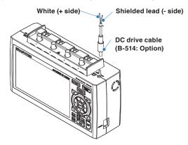
(3) Connect the DC input side to the DC power supply.
