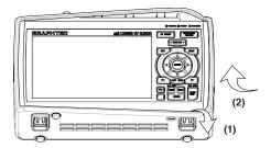
(3) When both corners of this device are removed from the Rubber Protector, pull the protector over the terminal block.
