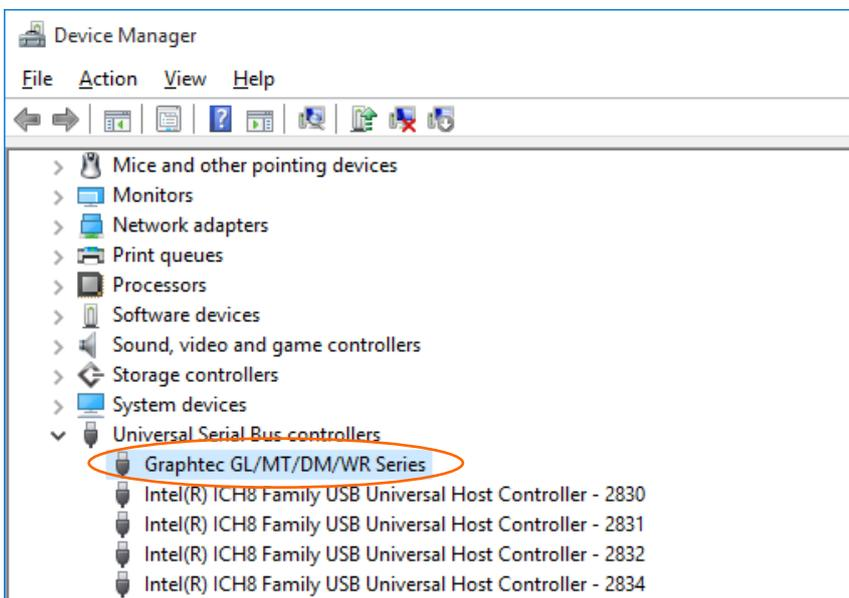
Confirm that the name of Graphtec GL/MT/DM/WR Series is registered and that there is no X or ! mark beside the name
