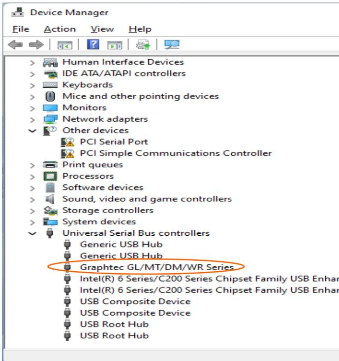
Confirm that the name of Graphtec GL/MT/DM/WR Series is registered and that there is no X or ! mark beside the name
