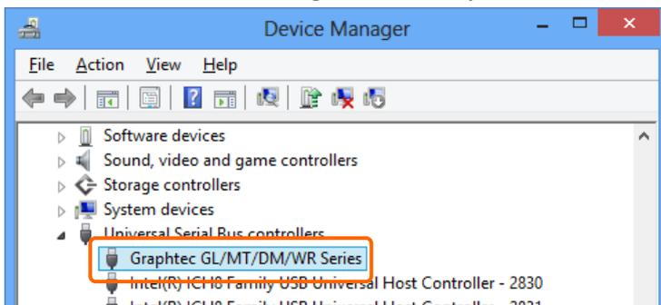
Confirm that the name of Graphtec GL/MT/DM/WR Series is registered and that there is no X or ! mark beside the name
