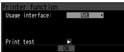
Select [USB] for [Usage interface] on [Printer function]. The printer is additionally displayed on the upper right of the menu screen.
