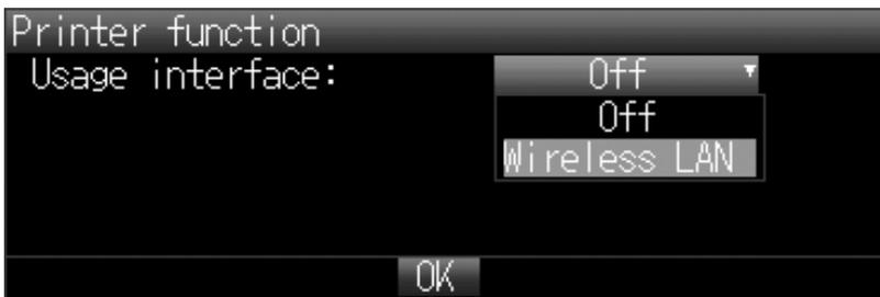
By selecting [Wireless LAN] on [Printer function], [PRN] is added on the menu.
