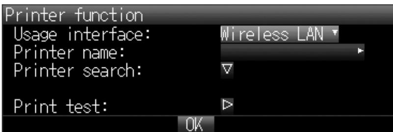
When wireless LAN is selected as the interface to be used, enter the printer name directly or search for the printer to be connected.
