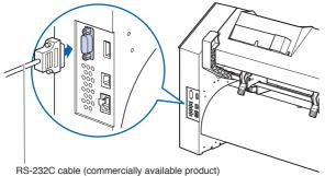
(9-pin female - 9-pin female straight connected cable)
