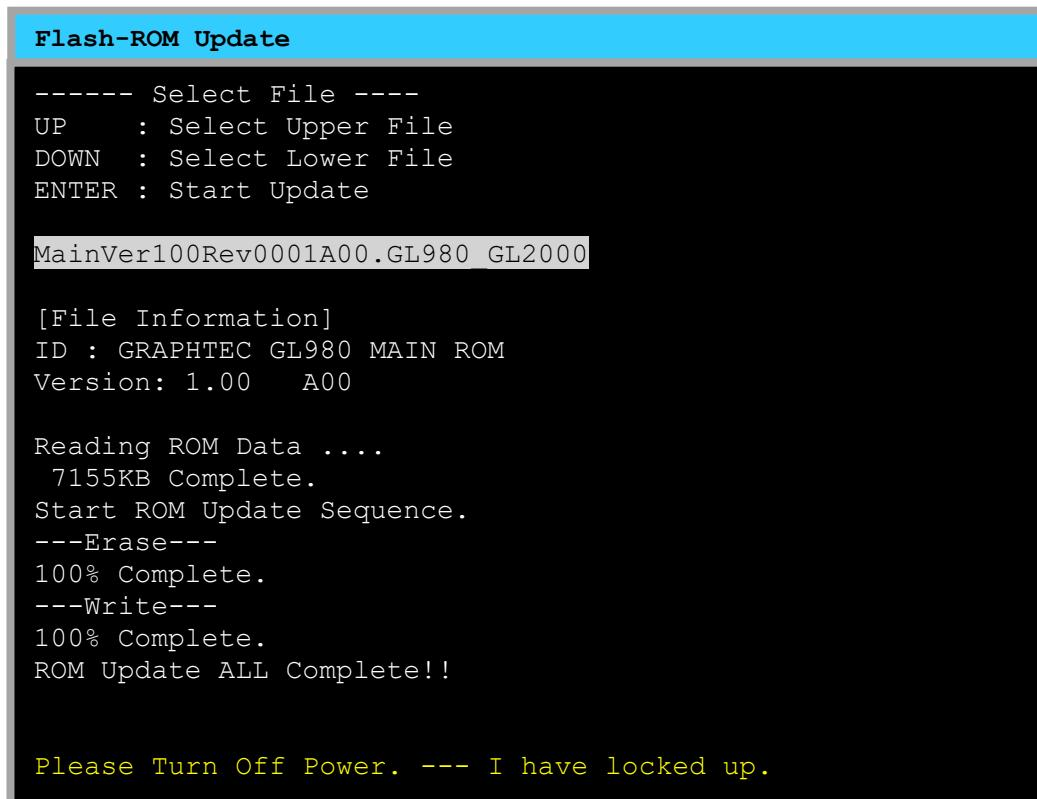
(4) Remove the media that has used for updating and turn on the power.
