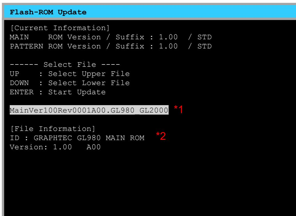
\*1 The file name is the name of the upgrade file prepared in step "2-3 Preparation for Version Upgrade". One of the two corresponding upgrade files will be displayed depending on the unit you use.
