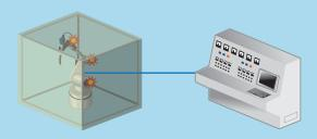
The malfunction of the control device is life-threatening. Tests under various radio wave environments that may induce malfunctions are required. e.g. Robot, Actuator, ECU
